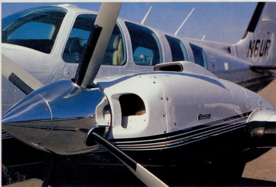
This 1980 Baron 58 underwent the full Foxstar treatment, including new four-blade Q-Tip props and new nacelle inlets (left). Zip-Tip winglets (facing page) add 20 inches to the wingspan, boosting the Baron's single-engine service ceiling to 10,000 feet.
