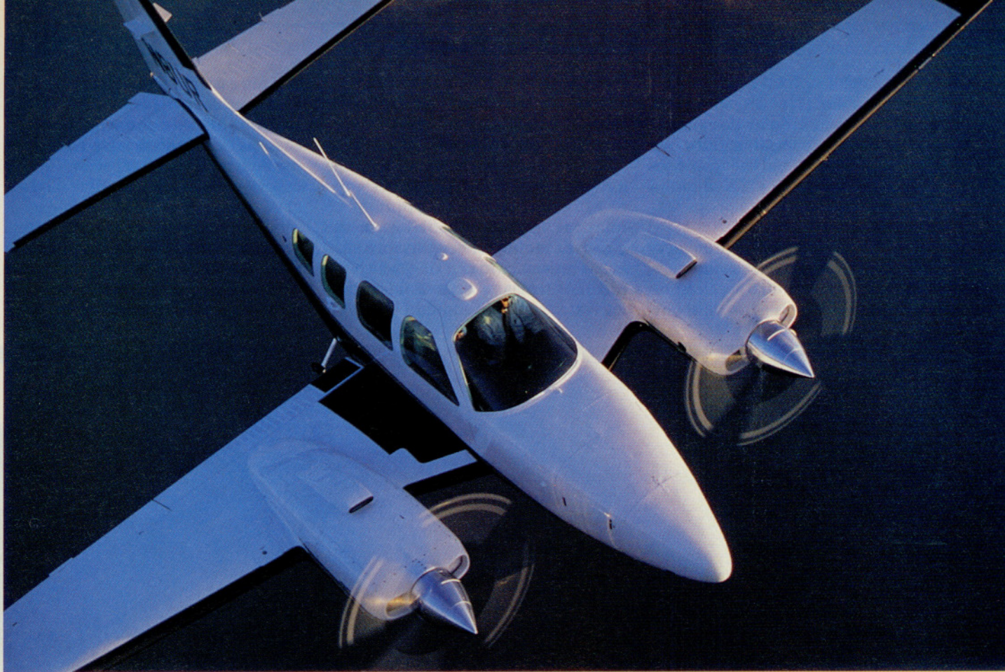
This 1980 Baron 58 underwent the full Foxstar treatment, including new four-blade Q-Tip props and new nacelle inlets (left). Zip-Tip winglets (facing page) add 20 inches to the wingspan, boosting the Baron's single-engine service ceiling to 10,000 feet.
